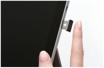
Match-in-Sensor™ Fingerprint Technology — Exceeds industry standards for False Rejection Rate (FRR 2%) and False Acceptance Rate (FAR 0.001%). Fingerprint data is secured in the sensor, so only an encrypted match result is transferred; versus match-on-host, where unsecured fingerprint data is transferred.
