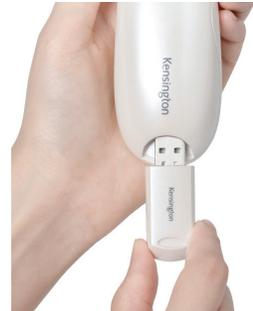
**Internal receiver storage** provides a convenient place to store your wireless USB receiver so it won't get lost, as each presenter and receiver are uniquely paired to prevent interference.
