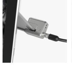
Non-Invasive Locking Technology provides an easy-to-use security solution that requires no device modifications, preserving the Surface Pro and Surface Go hardware warranty and aesthetics.
