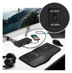
**Dynamic Video Support** through the docking station's dynamic 4K switch allowing you to toggle between modes, prioritizing resolution over USB, Ethernet, and SD Card speeds.
