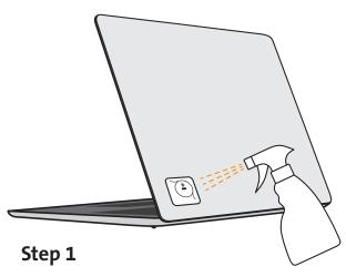
Apply a generous amount of adhesive remover around the slot adapter ensuring not to get the solution onto any sensitive components or areas of the device.
