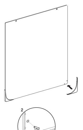
2. Attach each corner cap with (2) no. 6 x 1/4" screws.
